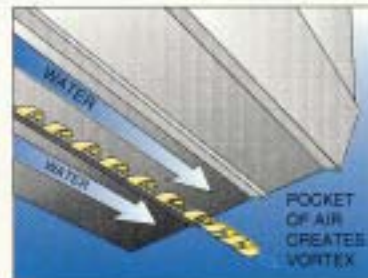
The patented "z-plane" hull is revolutionary in its reduction of air pockets and it's ability to integrate the new strakes into the hull for superior handling and agility. A notched transom allows the engine to be mounted higher thus reducing drag and increasing speed.
