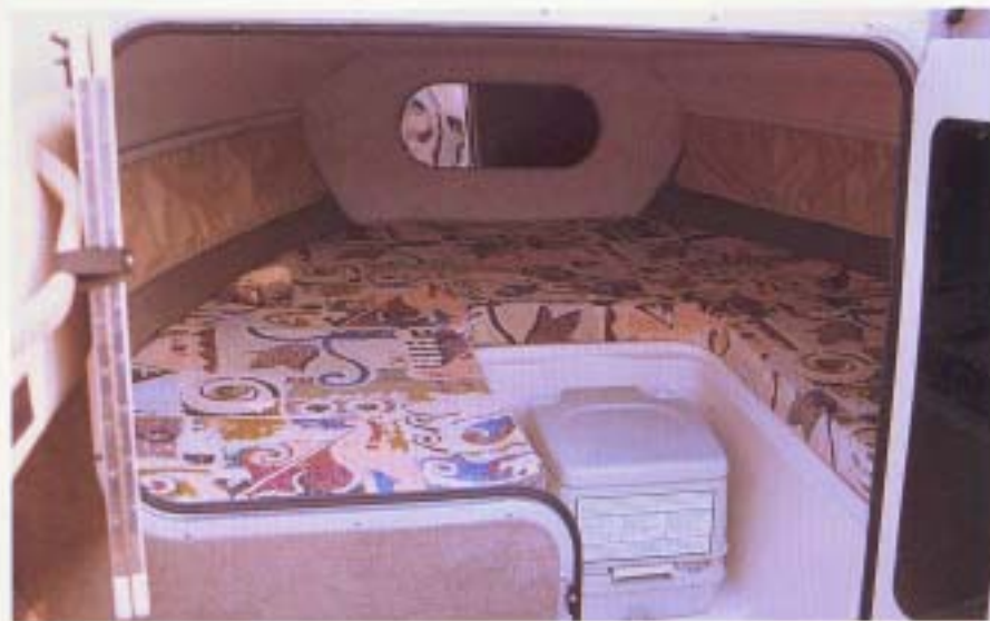
Molded Fiberglass Cabin Liner with Porta-Potti
