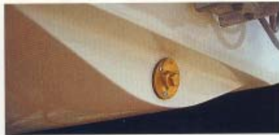
Brass Garboard Screw-in Drain Plug
