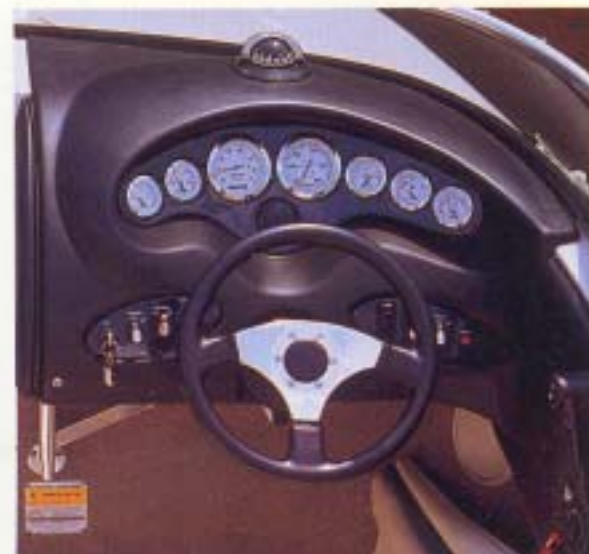
Custom Backlit Instrumentation with S/S Bezels
