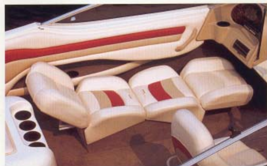
Adjustable Lounge Seats with Injection Molded Polypropylene Cores
