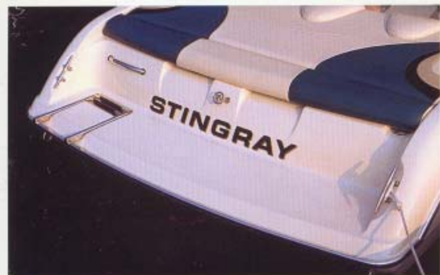
Integrated Swim Platform with Thru-Bolted Transom Hardware and Recessed Cleats and Ladder
