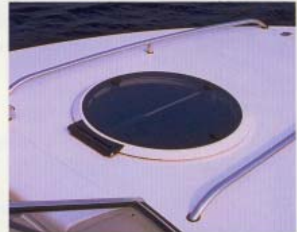
Translucent Aluminum Frame Deck Hatch
