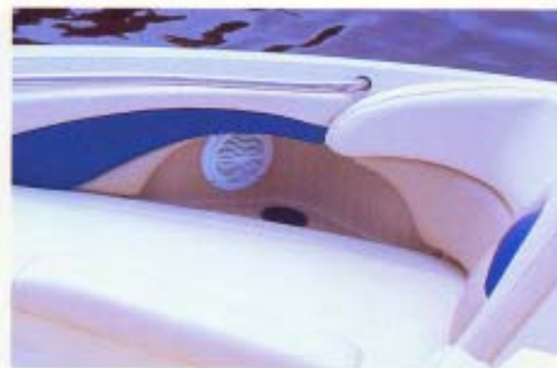
Molded Coaming Insert with weatherproof speakers and drink holder
