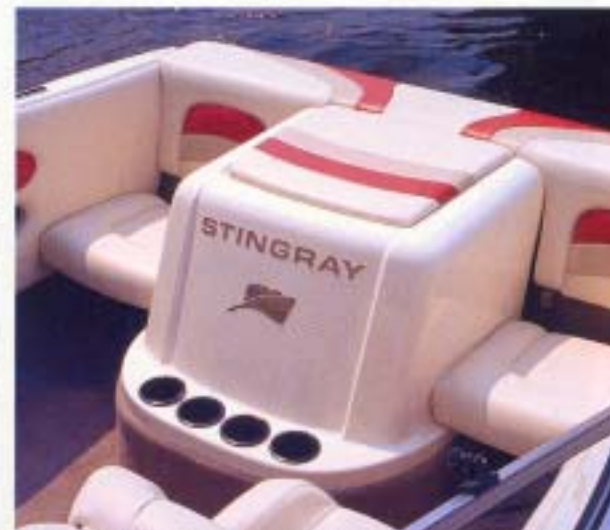
Fiberglass Insulated Motor Box with Upholstered Pad
