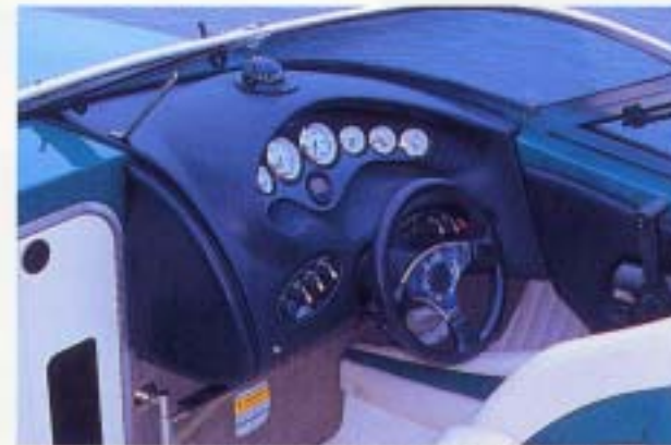
Custom Dash with Backlit Instrumentation, S/S Bezels, and Tilt Steering with Custom Wheel
