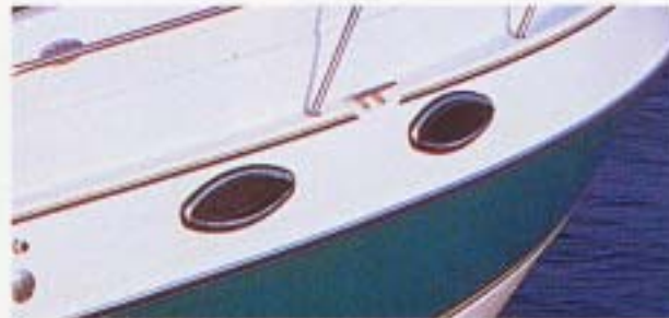
Opening Stainless Steel Port Windows
