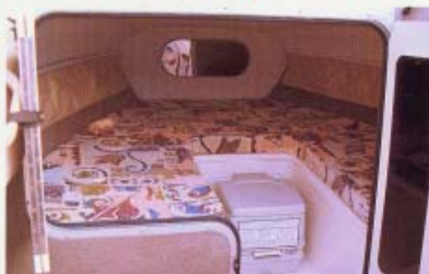
Molded Fiberglass Cabin Liner with Porta-Potti
