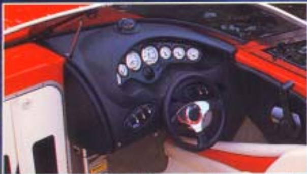
Custom Dash with Backlit Instrumentation, S/S Bezels, and Tilt Steering with Custom Wheel
