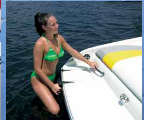
Integrated Swim Platform with Thru-Bolted Transom Hardware and Recessed Cleats and Ladder
