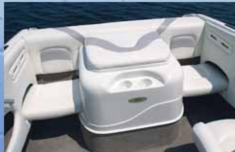
High Low Jump Seats (LS & CS Models Only) Insulated Fiberglass Motor Box with Upholstered Pad
