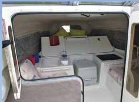
Molded Fiberglass Cabin Liner with Sink, Butane Stove, and Porta-Potti
